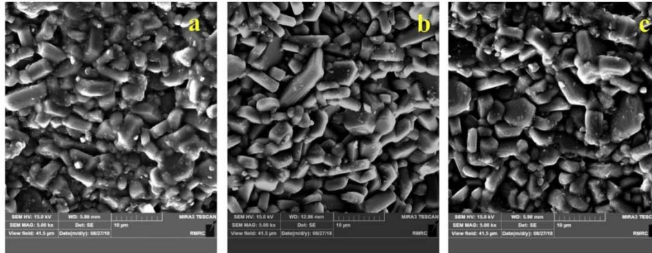
Fig. 7. FESEM images of samples with different amount of TMAH (wt%) a) 0.2 and b) 0.4 and c) 0.8.
